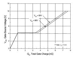
Figure 6. Gate Charge Characteristics
