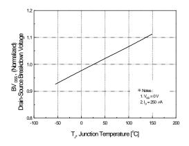
Figure 7. Breakdown Voltage Variation vs. Temperature
