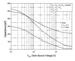
Figure 5. Capacitance Characteristics
