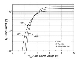
Figure 2. Transfer Characteristics
